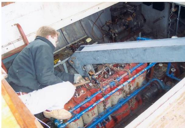
John attaching crane boom directly to the engine.
