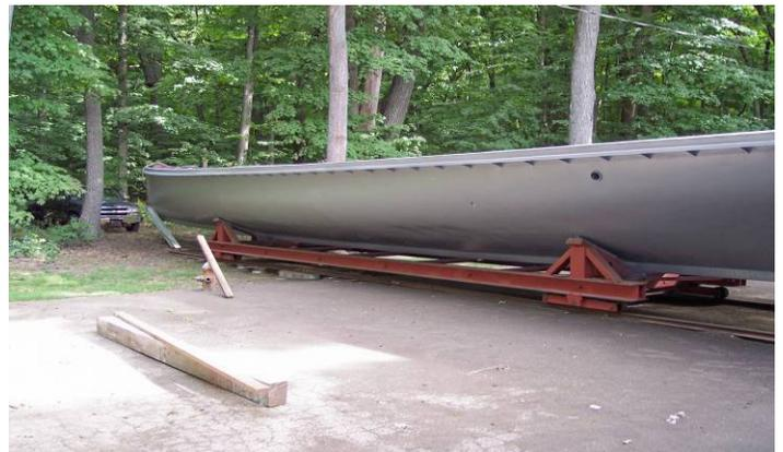
Exterior of hull sand blasted and painted with two coats of full immersion epoxy primer.
