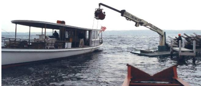
The engine is out of the boat, and the front end of the barge is almost under water.
